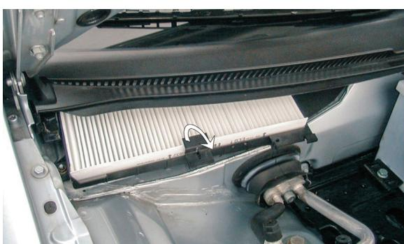
(EN) Remove the filter lock
