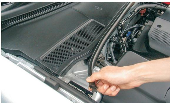
(EN) Remove the rubber seal
