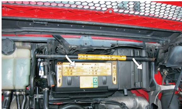
(EN) Remove the protecting device
