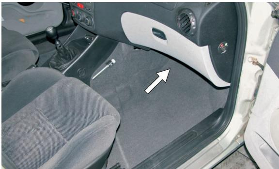
(EN) The filters are located under the glove compartment
