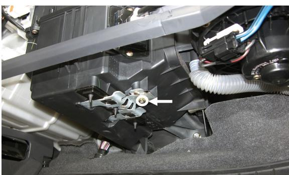
(EN) Unscrew the screw fastening the element shown on the picture
