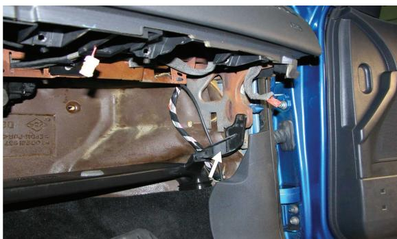
(EN) Remove the protecting device
