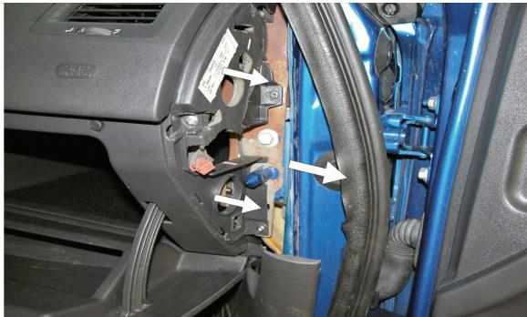
(EN) Remove the rubber seal. Loosen the screw and remove the upholstery panel
