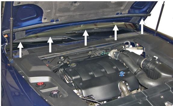
**(EN)** Carefully detach the screen under the windshield without damaging the sprinkler tube
