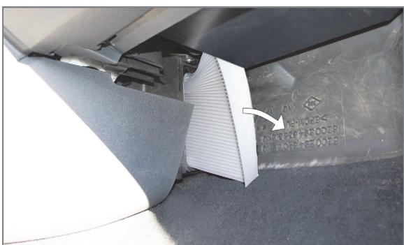
(EN) Gently remove the old filter, put in the new one and close the cover of the filter chamber attached in the kit
