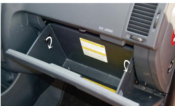
(EN) Remove the glove compartment
