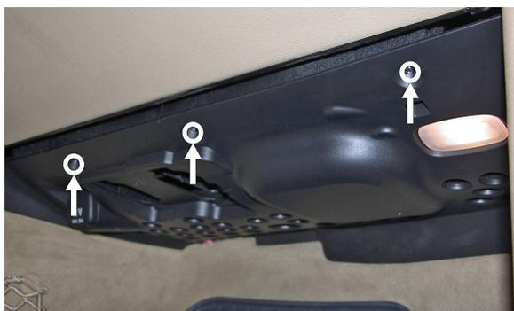
(EN) Loosen the screws and remove the upper wall of the locker
