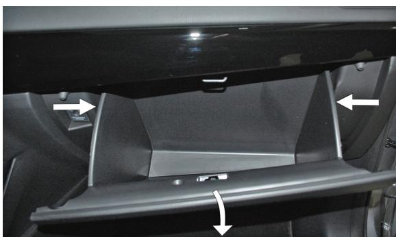
**(EN)** Remove the glove compartment
