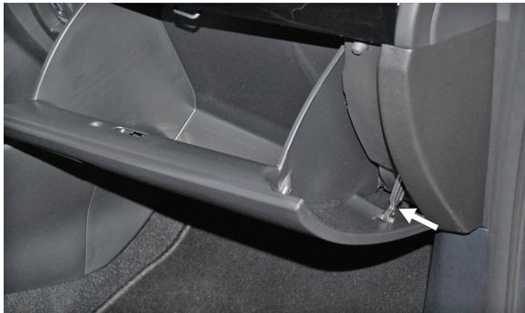
**(EN)** Remove the protecting device
