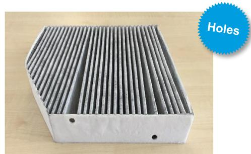
**Image 2:** The OE filter has two holes. Two pins placed in the housing can ingress in the filter.
